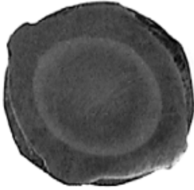
Fig. 3. Macrostructure of the strengthened reinforcing rolled stock with a diameter of 12 mm of grade A500S.
